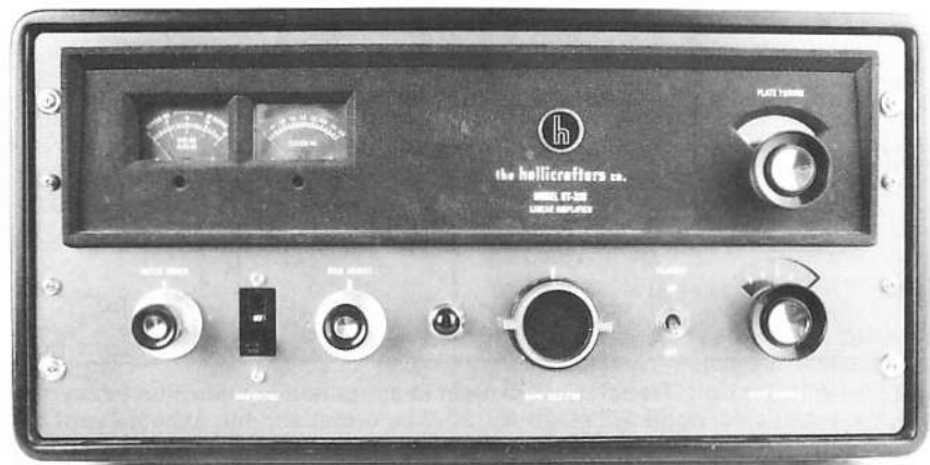
Fig 22.49 —Typical of ham gear from the 1950s and early '60s, this classic Hallicrafters HT-33B Linear Amplifier features a 117 V ac plate transformer. The magnetic circuit breaker on the front panel trips at a line current of 22 Amps! Many existing 110 to 120 V ac branch circuits would be unsuitable for such a load.
